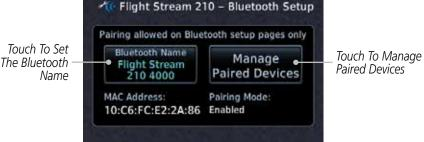
Figure 15-64 Bluetooth Setup for Flight Stream 210
