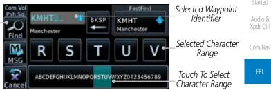
Figure 4-5 Select a Waypoint for the New Flight Plan
