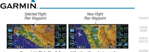
Figure 4-14 Flight Plan Before and After New Waypoint Inserted
