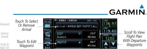
Figure 6-14 Flight Plan With Arrival Loaded
