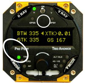
This indicates that the roll servo has been activated by pressing the **H NAV** button and the Pro Pilot is providing horizontal navigation, having taken control of the roll axis of the aircraft.
