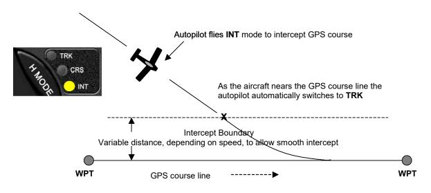
In both the **CRS** and **INT** mode, the ground track heading may be changed by rotating the encoder knob or using the **PCS** steering mode of operation.
