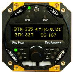
The track mode (**TRK**) is used to track a GPS flight plan or fly directly to a "GOTO" waypoint. The autopilot uses the data stream from the GPS for determine the direction of flight. This mode requires a valid GPS signal to provide position information. If no GPS signal is present, this function will not be available.
