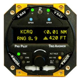
Since the **GPSV** does not function without the **GPSS**, the **GPSV LED** will also flash once per second, and vertical guidance will be controlled by the front panel of the Pro Pilot.
