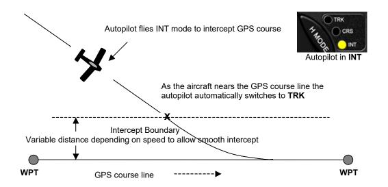
The automatic transition from the **INT** mode to the **TRK** mode is a function of the **XTK** (crosstrack error) magnitude, which is an index of the difference between the original course line and the position offset from the course line.
