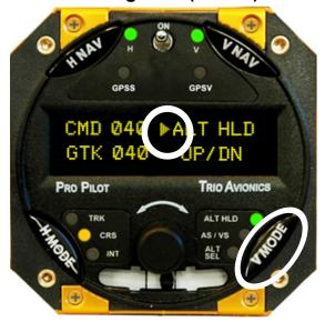
Generally speaking, except for warnings and alerts, the display screen will present the Vertical Navigation information on the righthand half of the display screen when the encoder has been assigned to the **VNAV** functions.
