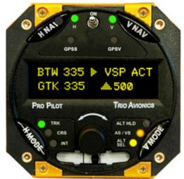
To work properly, the Pro Pilot must start with accurate altitude information. Once the pilot has adjusted the baro setting on the aircraft altimeter, the **ALTITUDE** setting in the Pro Pilot may be easily adjusted to agree with the aircraft altimeter by repeatedly pressing the **V MODE** button to display the **ALTITUDE SET** screen and changing the altitude setting by rotating the encoder knob.
