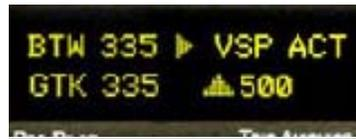
4. The autopilot will capture the vertical speed (VS) or airspeed (AS) that was programmed prior to flight.
