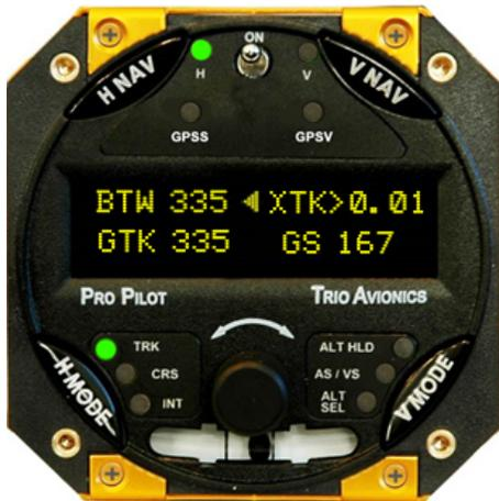
The track mode (**TRK**) is used to track a GPS flight plan or fly directly to a “GOTO” waypoint. The autopilot uses the data stream from the GPS to determine the direction of flight. This mode requires a valid GPS signal to provide position information. If no GPS signal is present, this function will not be available.
