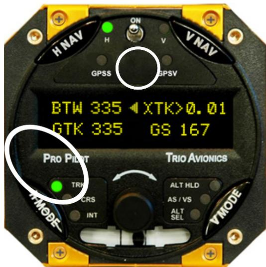
This indicates that the roll servo has been activated by pressing the **H NAV** button and the Pro Pilot is providing horizontal navigation, having taken control of the roll axis of the aircraft.
