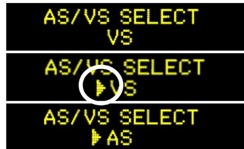
The **AS/VS SELECT** procedure is complete and the encoder can now be used to select another menu screen.
